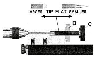
With electrode extending to the desired length, tighten the electrode wand. Loosen Nut D on the Tip Flat Gauge and insert electrode into the Tip Flat Gauge. Rotate Knob C until the Stop makes contact with the electrode tip, then lock in place with Nut D.
