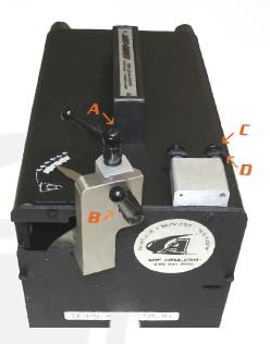
NOTE: Diamond Grinding wheels are specifically designed fo grinding tungsten electrodes only!
