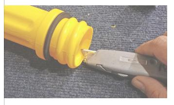
• Now lay the Rod Guard flat on a table and take you fresh utility knife or box cutter and slowly rotate the Rod Guard while firmly holding the knife. Try not to cut too much at a time, this will cause you to either remove too much material or create an unsafe situation.
