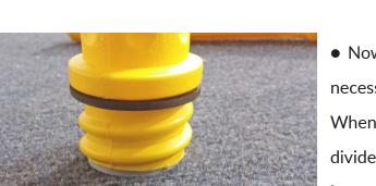
• Now test fit your divider again, remove more if necessary. You want to achieve a mild press fit. When there is enough clearance start pressing the divider into place. When the diver is <sup>1</sup>/<sub>3</sub> to <sup>1</sup>/<sub>2</sub> way inserted turn the assembly upside down then lightly press or tap it in place.
